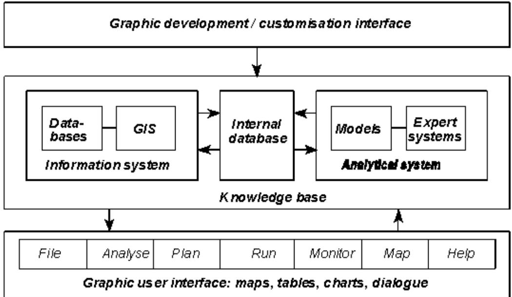
Figure 1 Architecture of the catchment modelling and analysis system
