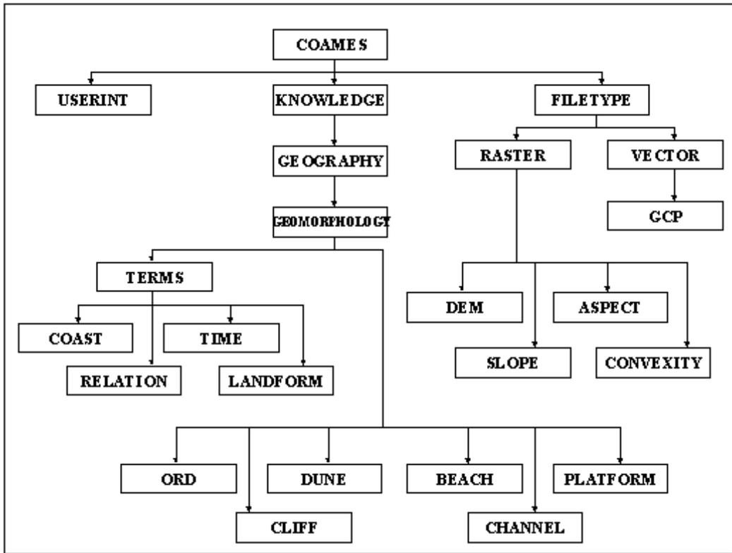
Fig. 6: The object-oriented hierarchical structure of knowledge and data in the COAMES prototype
