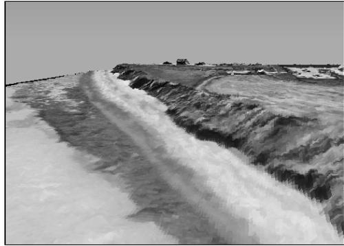
**Fig.4:** DEM covering part of Figure 3. The salient elements of the beach can clearly be seen, from the sand ridge on the left, through the darker till platform to the steeper upper beach banking the till cliffs.
