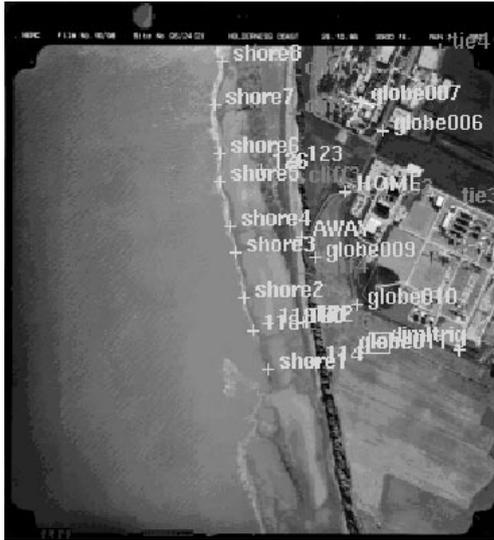
**Fig.3:** Aerial photograph of the Holderness coast near Easington with superimposed ground control and tie points. Taken 26/10/96.
