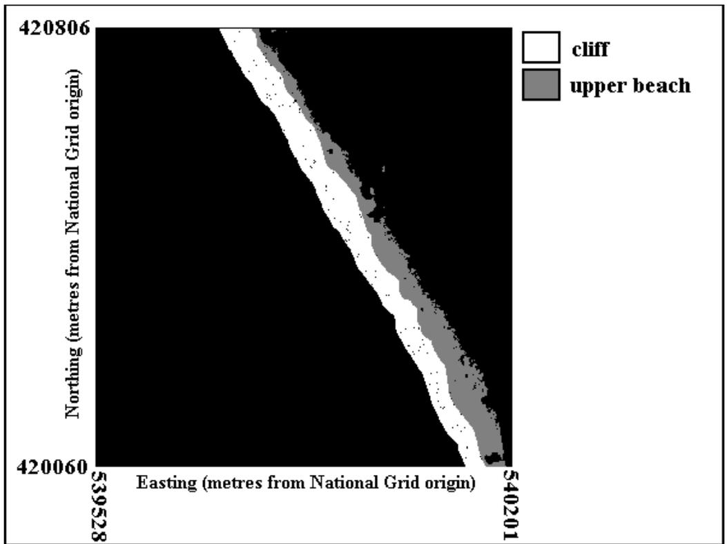
Fig.7: The isolation and extraction of the cliff and the upper beach from the study area on the basis of intelligent ground control points and morphometric parameters driven by the COAMES expert system
