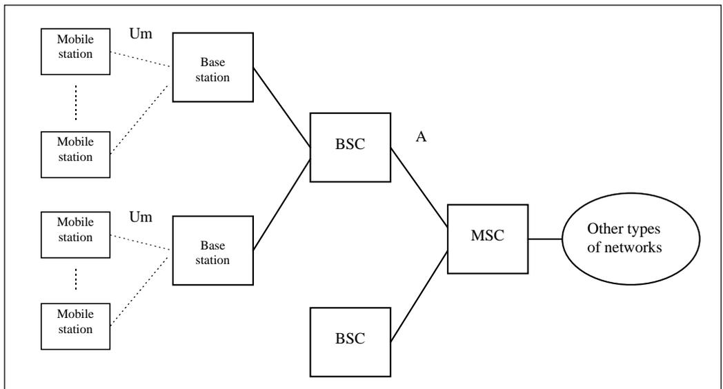
Figure 1. General architecture of a GSM network
