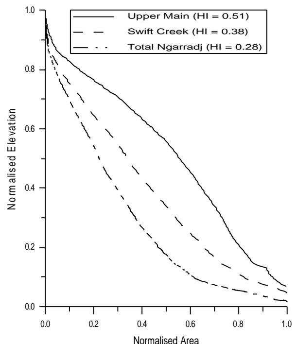
**Figure 2:** The hypsometric curves and integrals (HI) for the Upper Main, Swift Creek and Total Ngarradj catchments.
