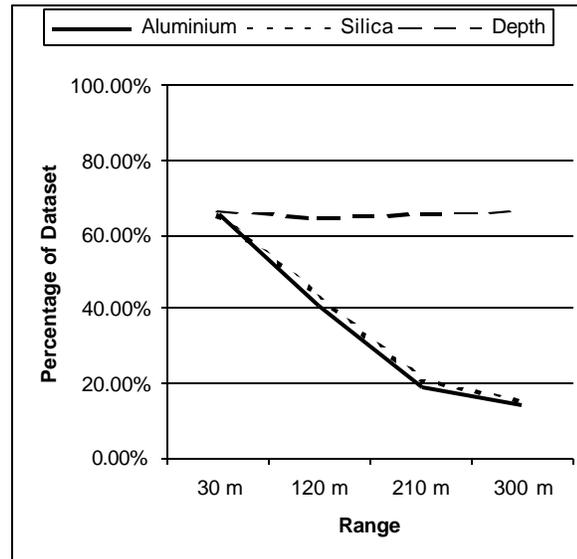
**Figure 3:** Proportion of sample dataset (38,928 data points) where watershed sampling returns stronger  $G_i^*$  clustering than omnidirectional sampling.
