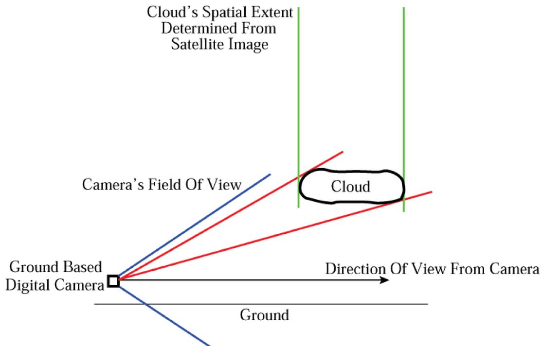
Figure 1, Simplified diagram of the relative perspectives of the satellite and digital camera images and how they can be used to produce 3D cloud models.
