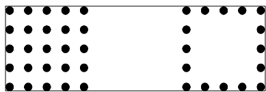
Figure 1. The number of grid points used by the sparse grid system (right) is much less than that used for the full grid system (left).
