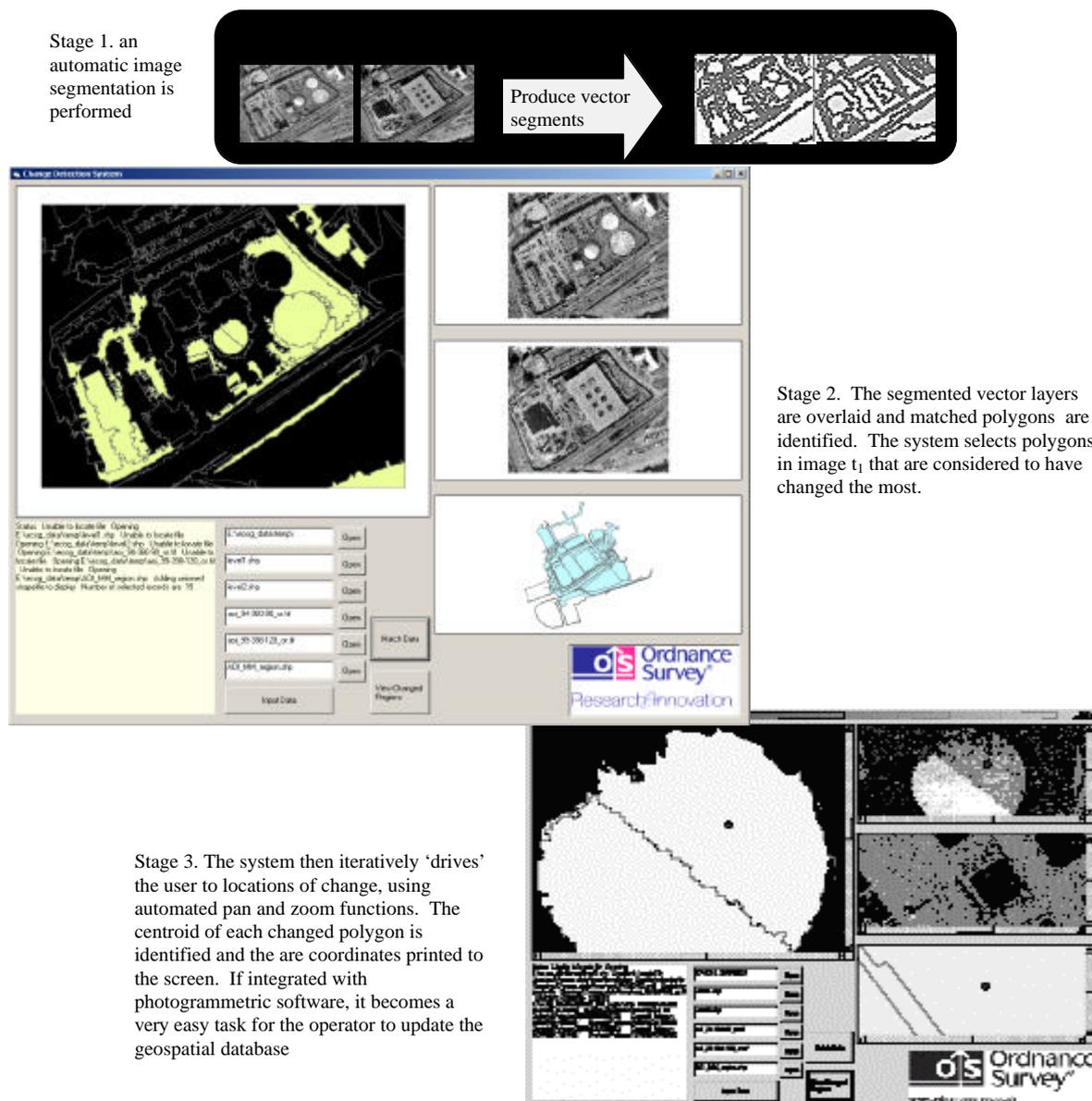
**Figure 3:** Process flowline through the prototype change detection system.
