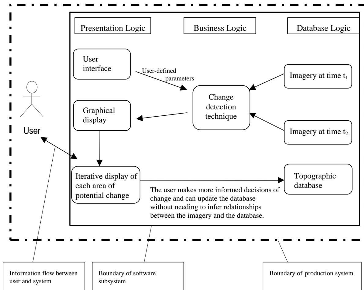
**Figure 2:** A tiered system design diagram illustrating the proposed change detection system within a data capture software environment.
