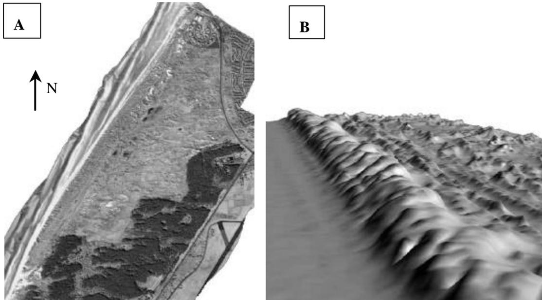
Figure 2. A: Band 12 (NIR) of the 1 m resolution CASI image of the Ainsdale Sands. B: 3D view of the 2 m resolution LiDAR DEM of the same area with the foredune clearly visible.
