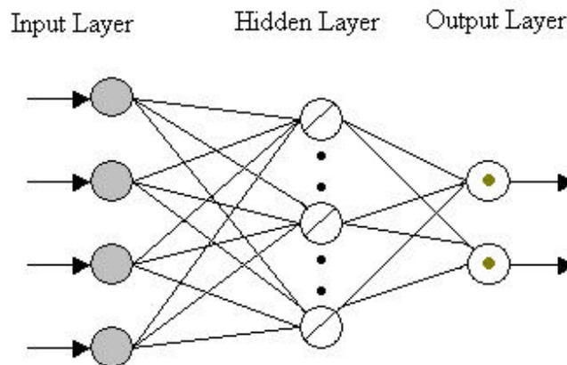
Figure 1. Schematic representation of a neural network with 1 input layer consisting of 4 nodes, 1 hidden layer with several nodes and 1 output layer with two nodes or classes (adapted from Lek and Guégan, 2000)
