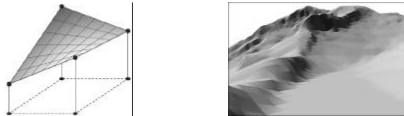
Figure 8. Bilinear interpolation. Right: bilinear surface patch. Left: globally C_0 -continuous surface composed of bilinear surface patches.
