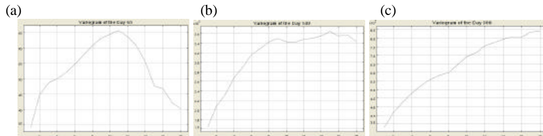
Figure 5 Variograms for days (a) 65, (b) 149 and (c) 308 showing some of the changes in spatial structure which occur through simulation runs.
