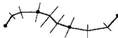
Figure 4: A stroke defined by 4 control points with intervening nodes generated by a cubic spline. The area covered by the stroke is approximated by quadrilaterals. (Strassmann, 1986)
