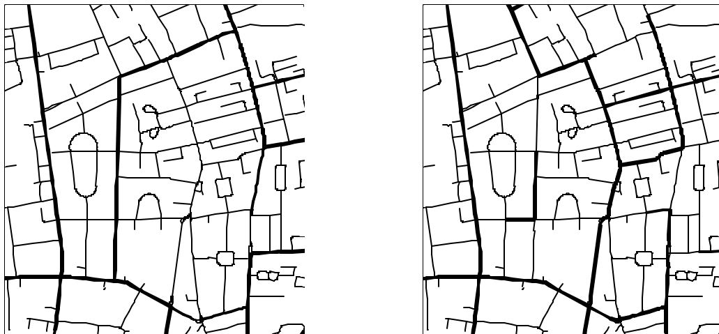
Figure 7. Left: Weighted betweenness ( B_w ) values for the minimum angular model at radius 2000m. Right: B_w values for the minimum block-distance model at radius 3000m
