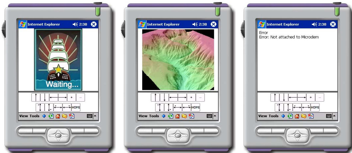
Figure 2. PocketPC screen captures connecting to MICRODEM via 3DPocketViewer shown in Figure 1. Controls on the bottom of the screen allow the browser to rotate and zoom the OpenGL block diagram.
