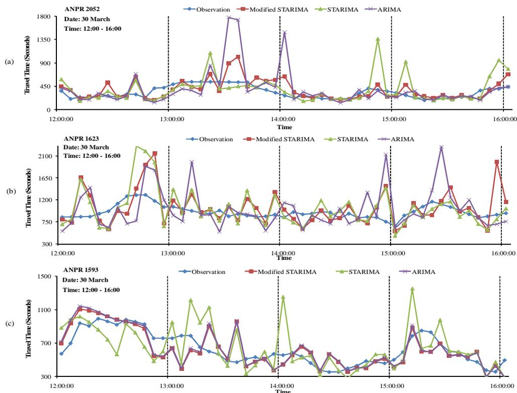
Figure 4. Prediction plots of three links 2052 (a), 1623 (b), and 1593 (c) at 12:00 - 16:00 on 30 Mar using three different models NSTARIMA, STARIMA, and ARIMA
