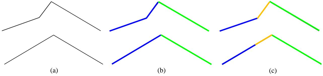
**Figure 2.** The establishment of corresponding vectors. (a) The original linear features. (b) The corresponding line segments obtained based on BLG-trees. (c) The corresponding vectors established based on the linear interpolation algorithm.
