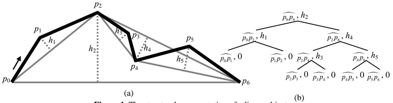
**Figure 1.** The structural representation of a linear object.
