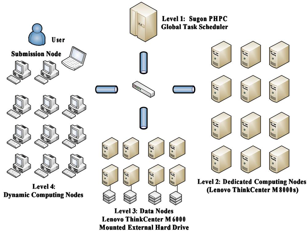
Figure 1. The physical architecture of the RSSN platform.
