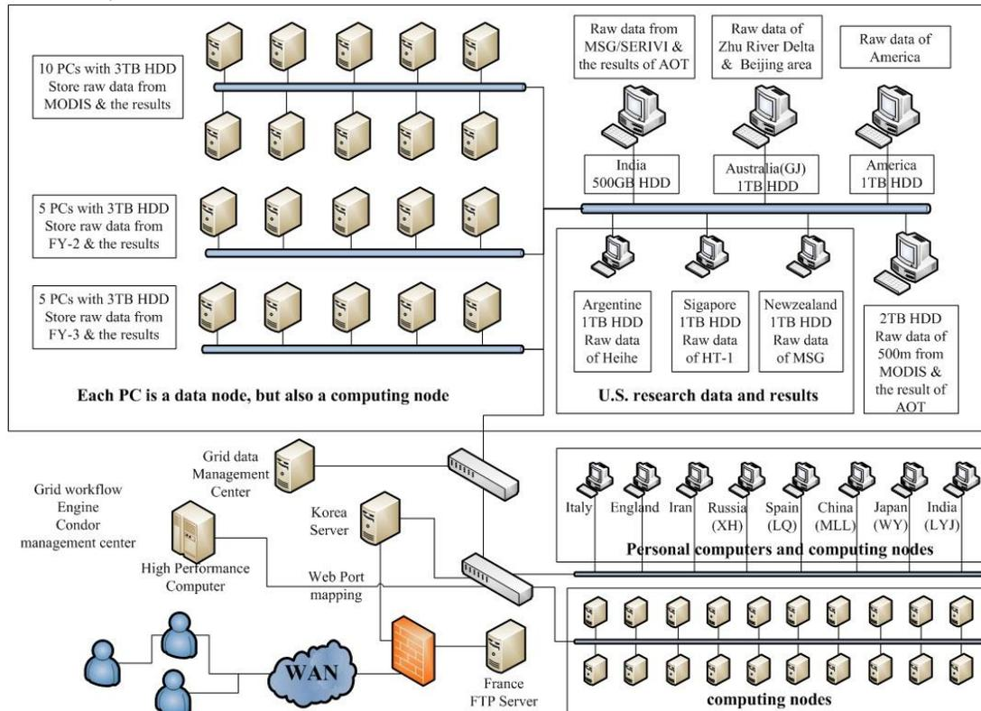
Figure 1. The physical architecture of RSIN system
