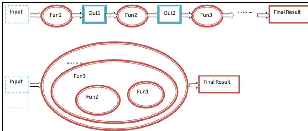
Figure 1. The generic frameworks of the traditional geo-processing method and Combinative Geo-processing.
