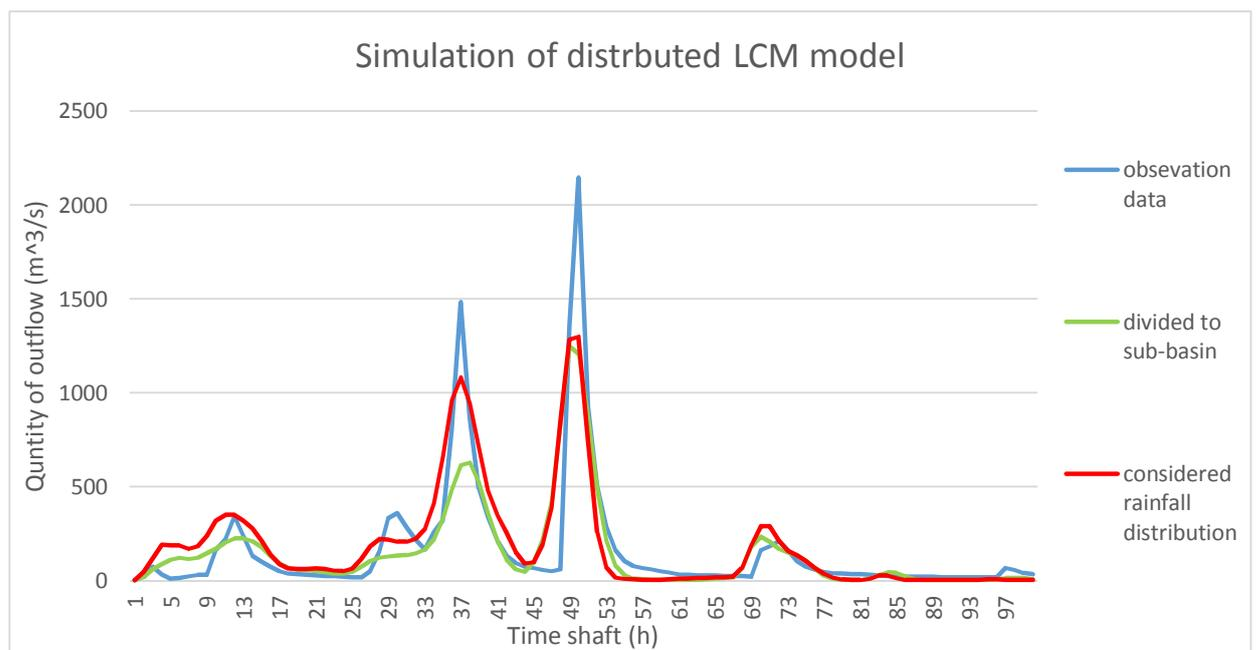
Figure.2 Continuous 100 hours outflow simulation in 1988, Gushanchuan
