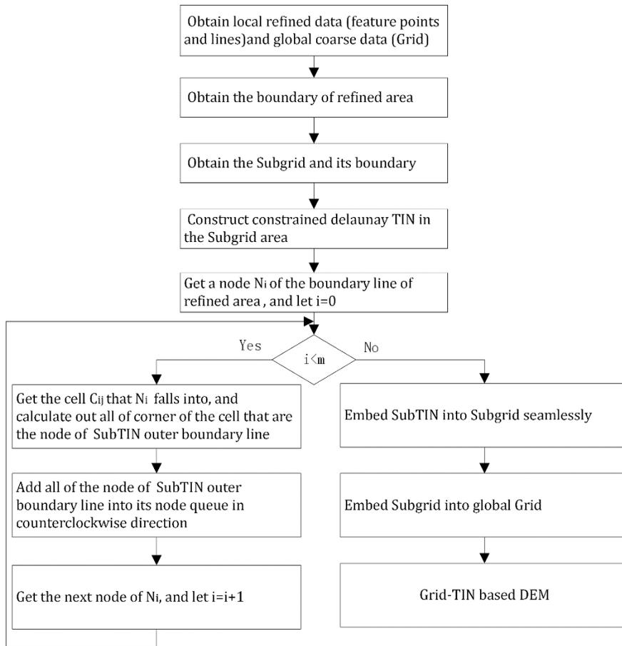
Figure 1. The technique flow of constructing a Grid-TIN DEM.
