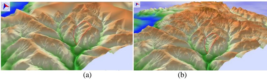
Figure 6. Visualization of (a) the 1:10,000 DEM; and (b) the Grid-TIN DEM in entire study area.
