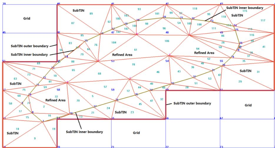
Figure 2. The relationship among the Subgrid, SubTIN and Refined Area in a Grid-TIN DEM.
