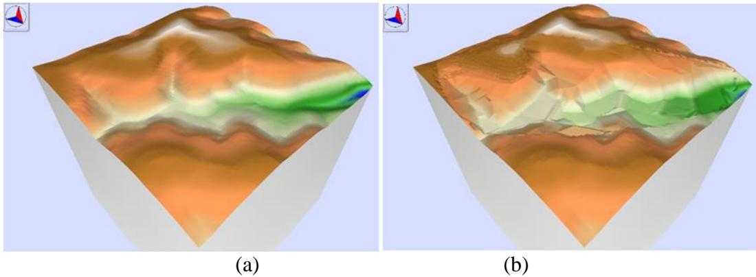
Figure 5. Visualization of (a) the 1:10,000 DEM; and (b) the Grid-TIN DEM in the scope of Subgrid.
