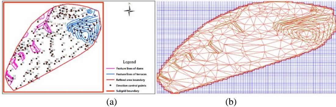
Figure 4. Distribution of (a) the feature points and lines; and (b) the hybrid mesh of the Grid-TIN DEM.
