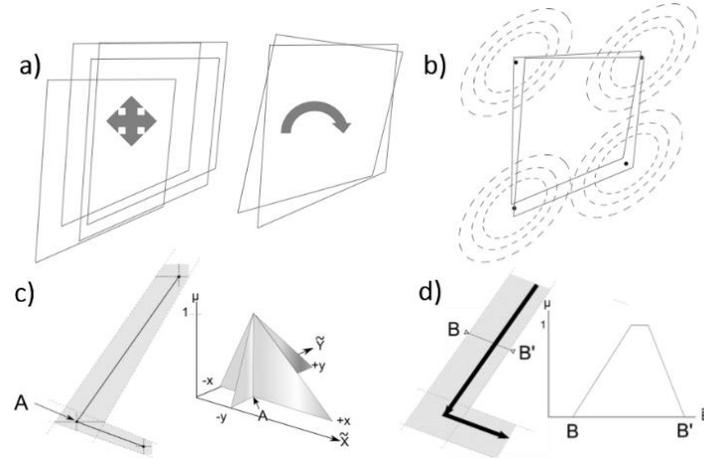
Figure 1: Uncertain objects. a) Rigid polygon, b) deformable polygon, c) vertex-defined polyline, d) edge-defined polyline. Adapted from (Rios 2014).
