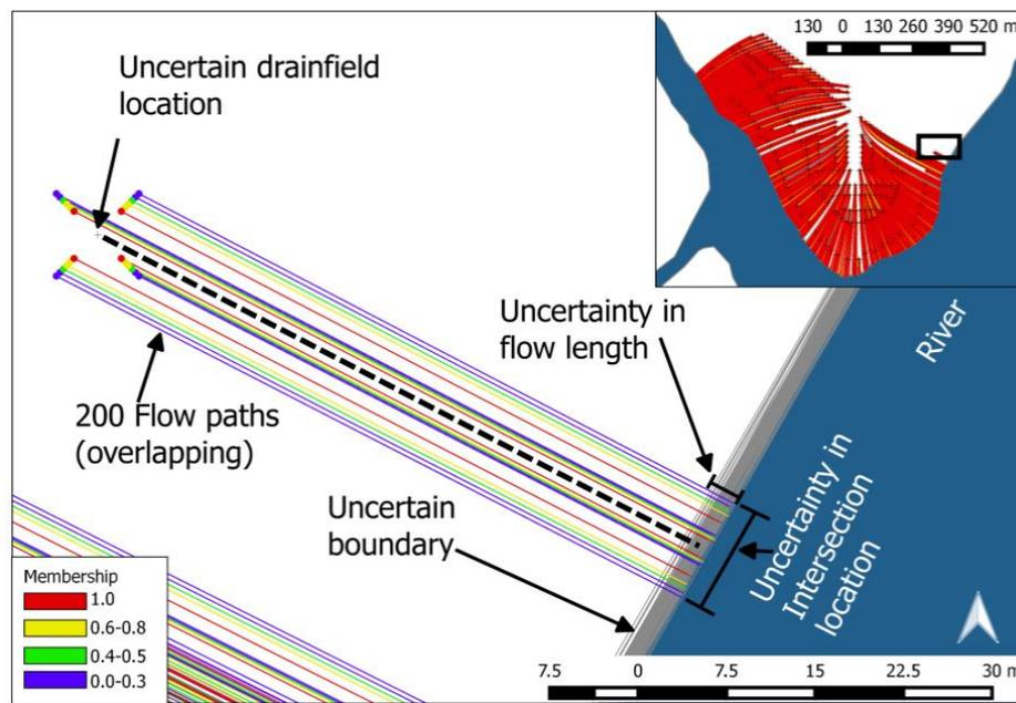
Figure 5: Effect of uncertainty on the flow path. Dashed line is the path without uncertainty. Note the 'X' shaped sampling of the drainfield location resulting from the reduced transformation method.
