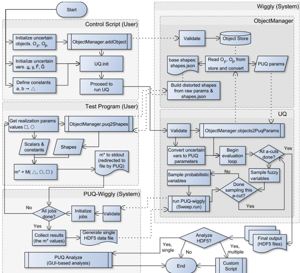
Figure 2: Implementation of the uncertainty conceptualization. The solid arrows indicate primary logic flow. Dotted arrows indicate transfer of flow to (or from) a subroutine. If the dotted arrows do not return, primary logic flow may continue without waiting for a return value. The dotted lines with no arrows indicates interaction between components, without transfer of flow.
