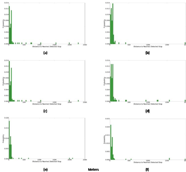
Figure 2. Probability Distribution of Collected Distances from Ground Truth Stops to the Nearest Detected Stops for (a) - (f) Methods.
