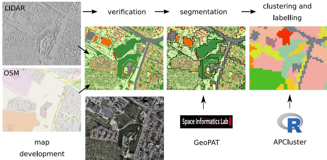
Figure 1: A data processing routine. From LIDAR cloud to Urban Structure Types
