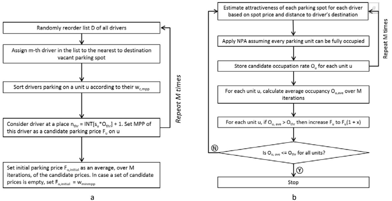
Figure 2: Two stages of the NPPA algorithm: (a) establishment of initial prices and (b) iterative increase of prices
