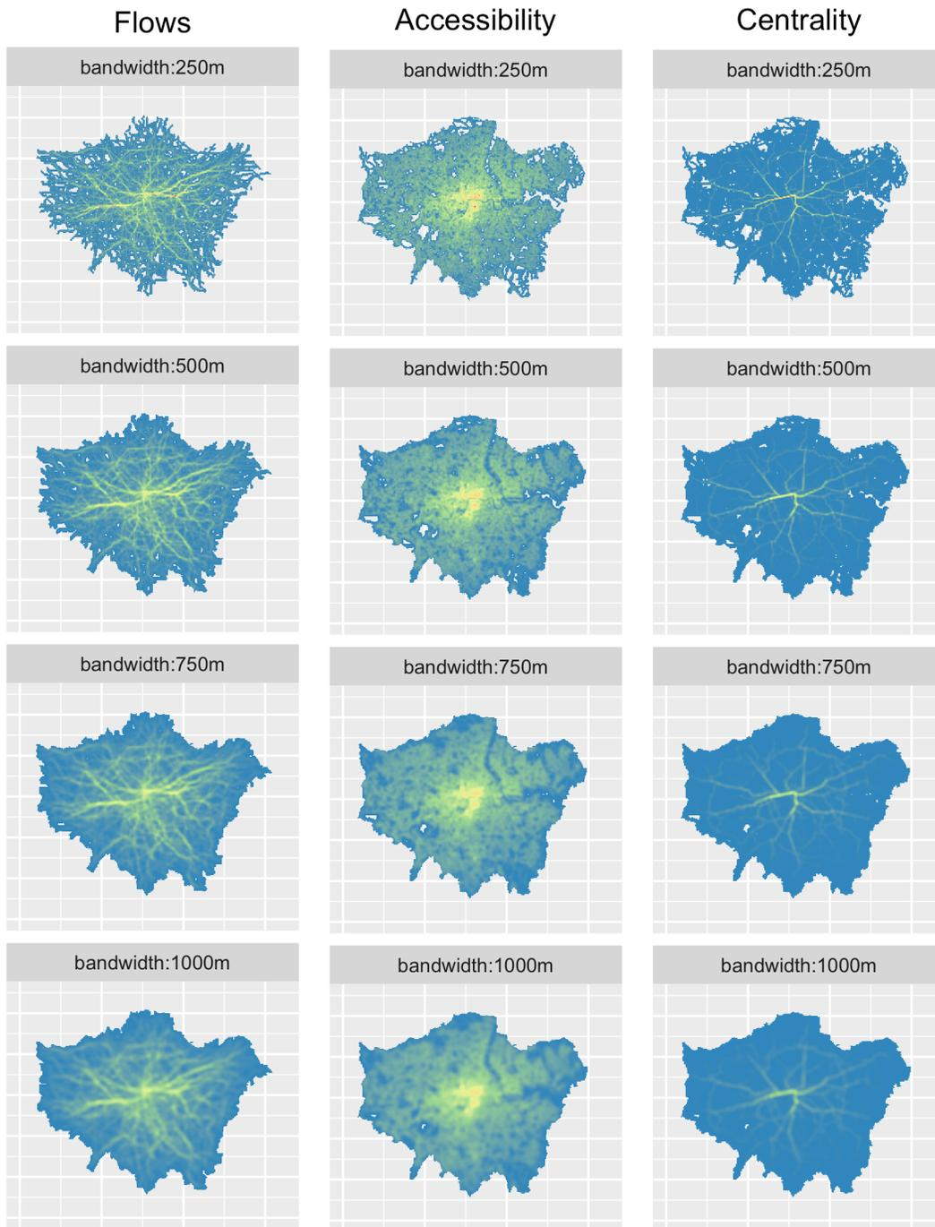
Figure 5 - Flows, accessibility and centrality densities calculated using the KDE method with four bandwidths.
