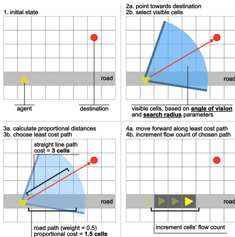
Figure 1 - Agents' walking procedure in the AXS model.
