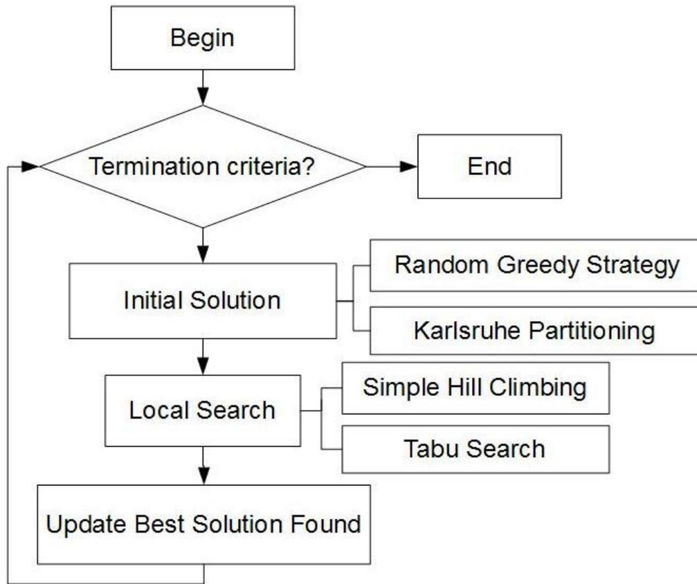
Figure 1. Flowchart of the algorithm for SNPDP
