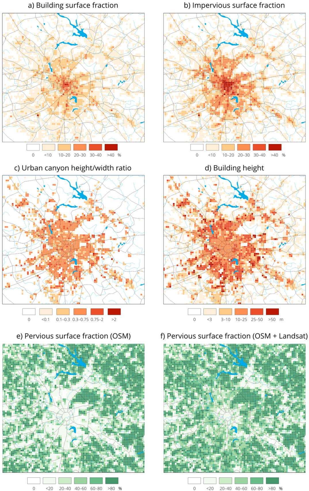
Figure 6: LCZ characteristics calculated from OpenStreetMap data (a-e) and OpenStreetMap/Landsat data (f).
